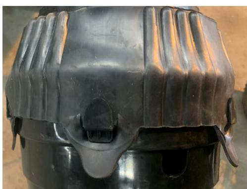
Pull on rubber tabs to release them from the plastic shroud and pull the rubber cover back. Grease zerks with 2 pumps as shown. Remember to grease all three cross bearings. The zerks are on the caps
